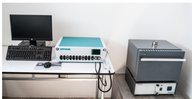
Figure 2 Corrosion tests by Electrochemical Impedance Spectroscopy.
