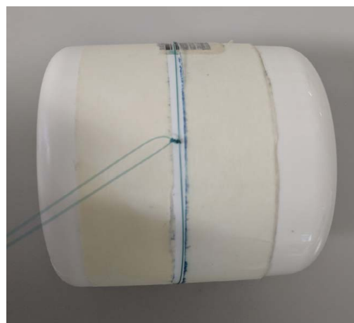
Figure 1. Suture loops created using a cylindrical template and secured with 8 reef knots.
