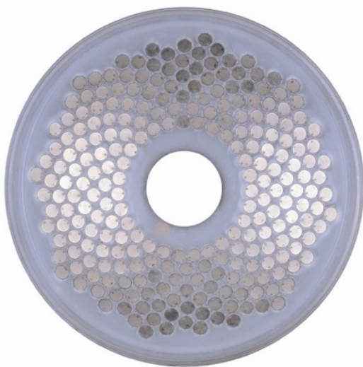
Figure 3. FEP-BY™ high intensity focused ultrasound transducer. The transducer is made of 251 individual piezoceramic elements and is concave with a geometric focus of 26 cm. The center hole in the transducer is for the ultrasound imaging probe. Reproduced with permission (Yuande Biomedical Engineering Corp. Ltd., Beijing, China).
