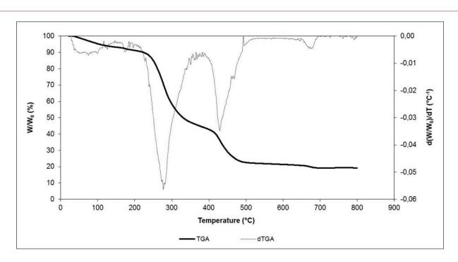
**Figure 1** Plot of percentage of residual sample weight, relative to starting sample weight (W/W<sub>0</sub>, %), and first derivative  $d(W/W_0)/dT$ , versus temperature (T,  $^{\circ}$ C). Data for raw 5-10 mm post-harvest tomato plant powder (PHTr).
